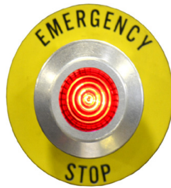
E-Stop activated. (LED illuminated)
