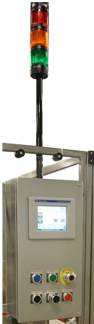
Figure 4-3. Main Light Stack
